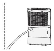
Make sure the connection between pipe and the drain outlet is tight and does not leak. Then direct the pipe to a suitable drainage point. This unit uses gravity fall to dispose water hence the drain should be lower than the unit water outlet. Put the tank back. Be sure to run the water pipe downward and let the water to flow out smoothly. Do not kink or bend the pipe.
