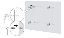
**Please note:** If drilling into tile, it is recommended to tape the wall to prevent the drill from slipping.
