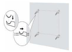
4. Once all brackets are secure, hang the radiator until fixed firmly into place and adjust so that the radiator aligns with the pipework.
