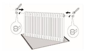
1. Mark the position of the wall hanging brackets (on the wall) on either side. Use a spirit level to ensure these are aligned.
