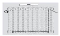
2. Using the drill and 8mm drill bit, drill into the marked positions then insert the wall plugs and tap flush to the finished wall surface.
