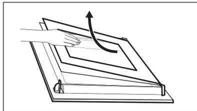
9. Clean the glass panel with water and soap. Dry the glass panel carefully. When the cleaning is completed, do the above steps in the opposite sequence. Install the smaller panel first, then the larger and the door.
