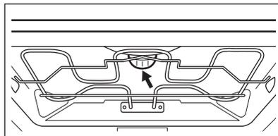
2. Remove the metal ring and clean the glass cover.
