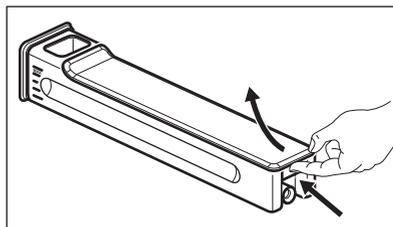
2. Remove the wave-breaker. Pull it away from the drawer body until it snaps out.
