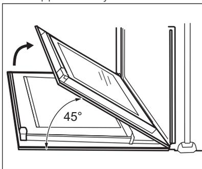
4. Hold the door with one hand on each side and pull it away from the appliance at an upwards angle.
