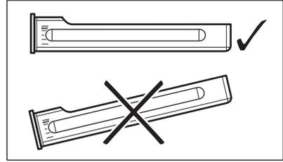
When you fill the water drawer, insert it in the same position. Push the front button until the water drawer is inside the appliance.
